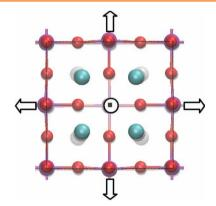
Computer simulations show that local relaxations around defect clusters explain the effect of rare-earth doping on the Curie temperature in BaTiO<sub>3</sub>. La and Gd induce similar relaxations, leading to distortion and tilting of the surrounding TiO<sub>6</sub> octahedra. Larger distortions are observed for La, consistent with the greater lowering of the Curie temperature.
