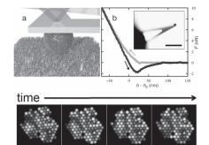
A simple method of rendering the interactions between nanoparticles thermosensitive using a thermoresponsive surfactant is described. The surfactant, based on poly(*N*-isopropylacrylamide) (pNIPAm), passively absorbs to surfaces, eliminating the necessity for chemical surface modification. This interaction and resulting self-assembly is investigated using colloid probe atomic force microscopy (CP-AFM), rheology, and confocal microscopy.
