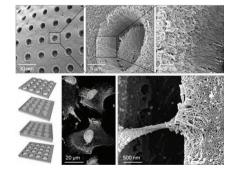
Hierarchically structured self-assembled membranes that incorporate both biomolecular and topographical signaling elements are fabricated in a single step process. The spontaneous co-assembly of hyaluronic acid and a multidomain peptide of opposite charge guided by microfabricated structures provides a simple method for producing a complex membrane scaffold for tissue engineering applications.
